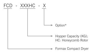
Note: \* DP= Dewpoint Meter HT=180°C High Temperature ES=Insulation Energy Saving Function P=Polish Internal Hopper
